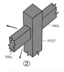
B) This system uses rails 100mm x 38mm in section and is nailed to the faces of the posts with 100mm flat head nails. See sketch 3a.
