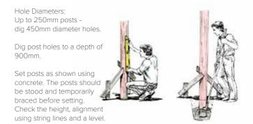
CONCRETE EMBEDMENT Use minimum 25mPa concrete for concrete footings
