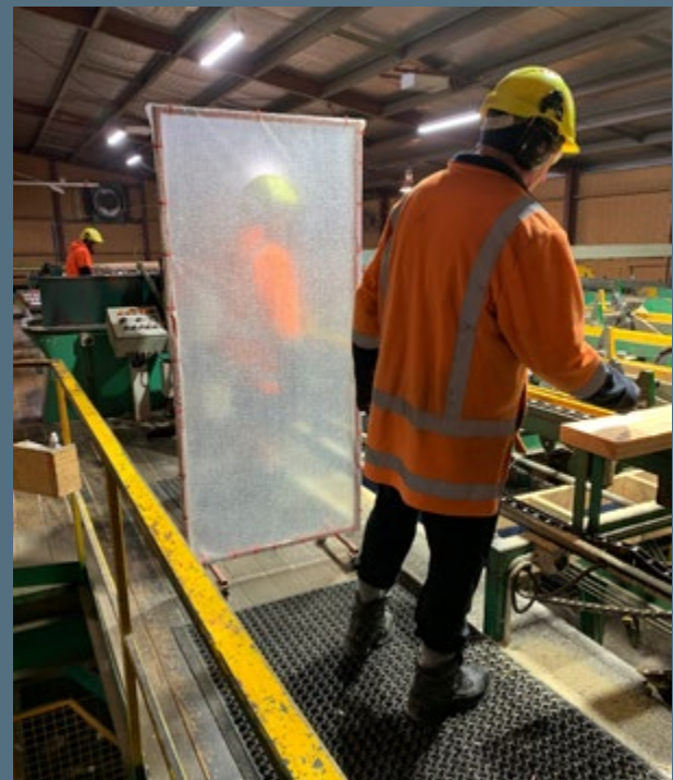
Grading area screen creating a safe barrier between operators
