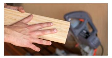
Dressed All Round (DAR) timber is finished in the mill to feel smooth to touch the whole way down. Microline or Rougher Header on the other hand has ridges carved down the length of the outside of timber.
