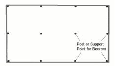
Lay the framing on concrete slabs bedded into position or on existing level concrete slabs.
