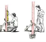
CONCRETE EMBEDMENT Use minimum 25mPa concrete for concrete footings
