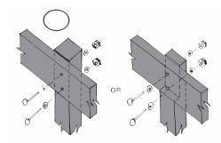
Fix joists to the bearers at max. 450mm spacing using triple grips or joist hangers, as shown in example below, and in accordance with manufacturers specifications.
