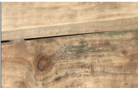
Examples of mould on new treated decking timber sampled from retail sites.
