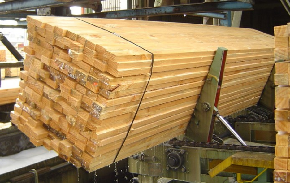
Example of an anti-mould chemical dipping operation to protect fresh timber from mould and stain
