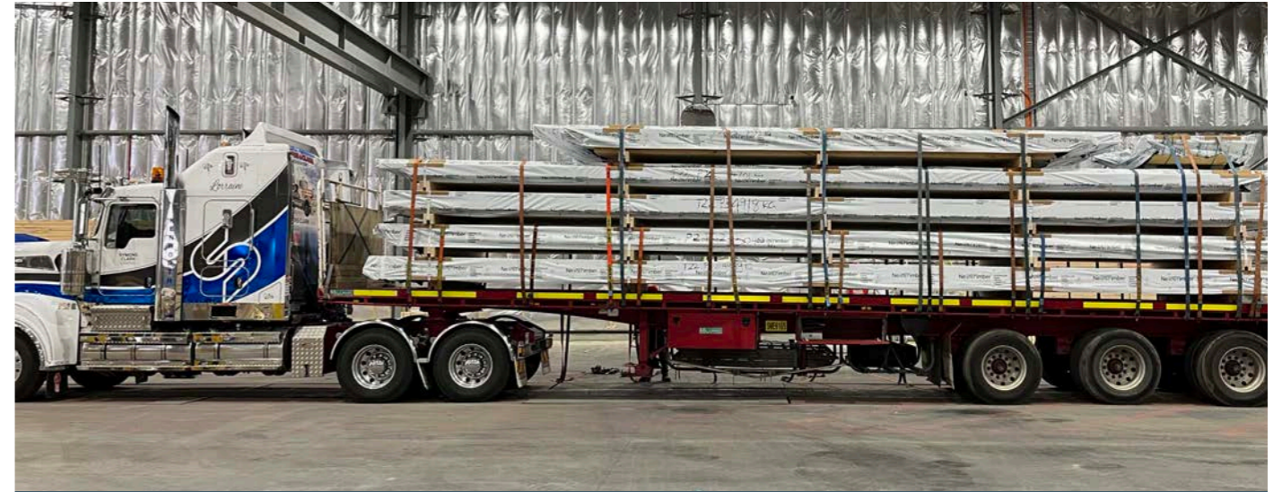
One of the 22 truckloads that delivered the nearly 200 individual CLT panels used to construct flooring and roofing for the Factory of the Future and Tonsley Technical College project.
